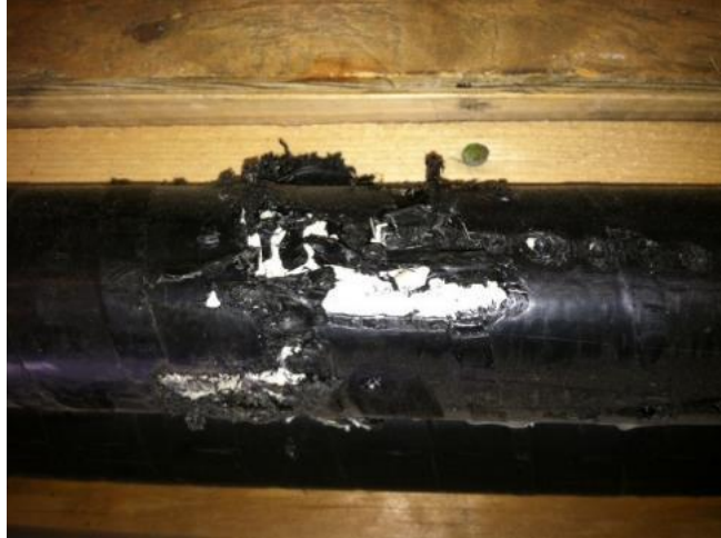
Fig. 4 Taped bar damaged in shipping
