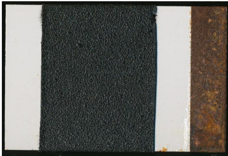
Fig. 21 Representative sample of Bonderite/53022/Dragonhide system at 30 cycles GMW14872
