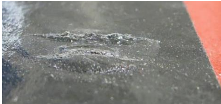
Fig. 18 Improved impact test on Line-X
