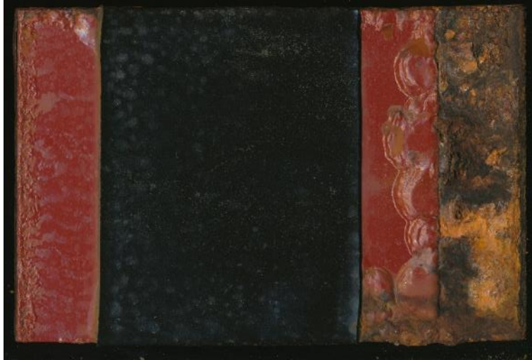
Fig. 22 Representative sample of XPM/Line-X system at 60 cycles GMW14872
