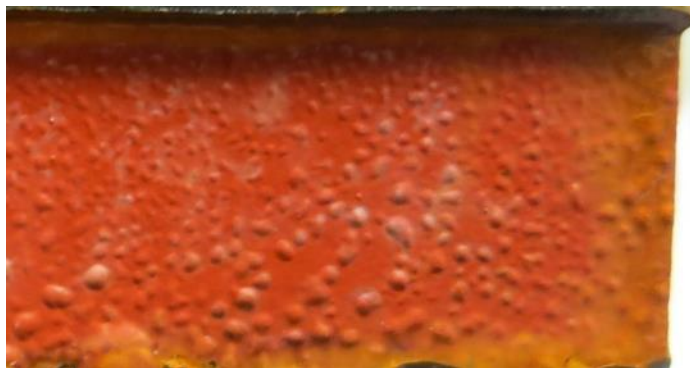
Fig. 24 Close up of blistering on XPM primed panels
