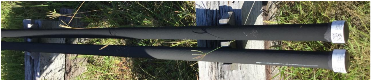
Fig. 30 Dragonhide (top) and Line-X (bottom) bars after 24 months of outdoor exposure at CCAFS
