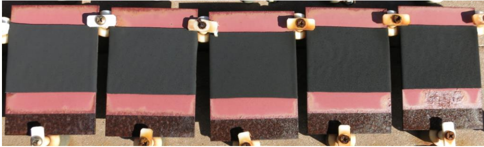
Fig. 28 Line-X system after 24 months of outdoor exposure at CCAFS
