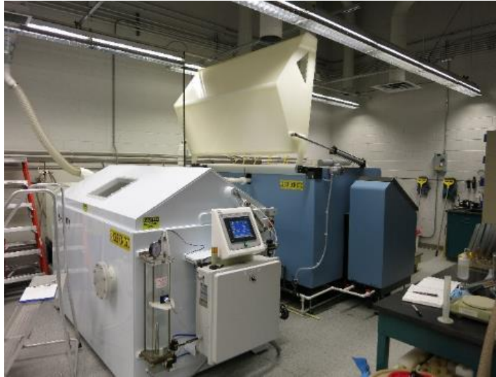
Fig. 6 Cyclic corrosion test chambers at ARL
