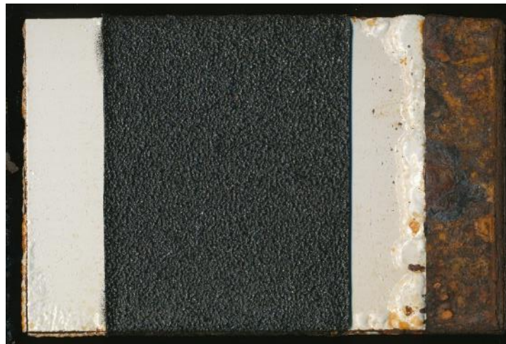
Fig. 23 Representative sample of Bonderite/53022/Dragonhide system at 60 cycles GMW14872
