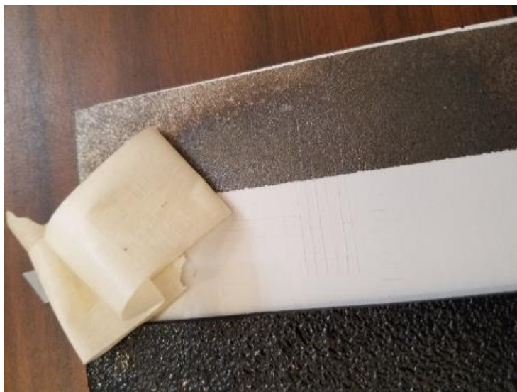
Fig. 12 Cross hatch on MIL-DTL-53022 type IV
