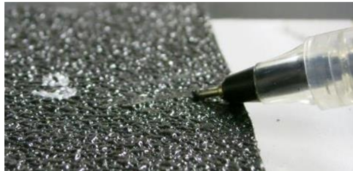
Fig. 19 Improved impact test on Dragonhide
