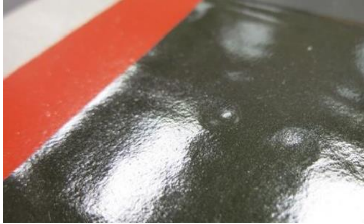
Fig. 15 Impact test results on XPM/Line-X System (left: 96 inch-lbs, right: 156 inch-lbs)
