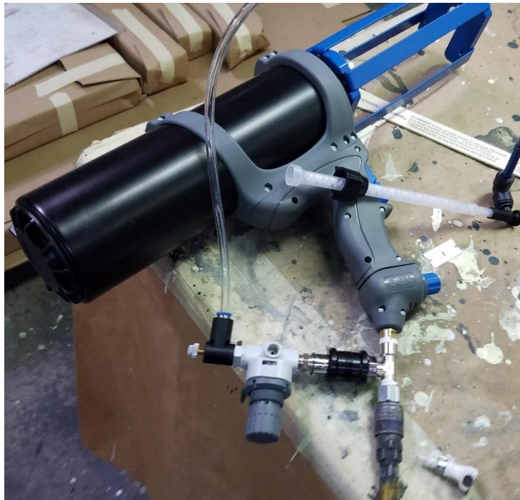
Fig. 10 Pneumatic dual cartridge epoxy gun setup
