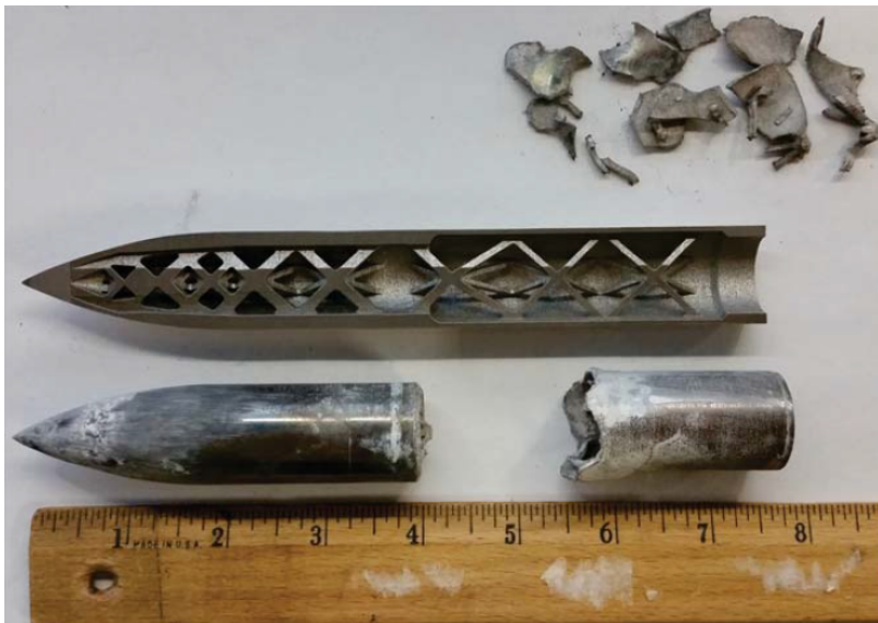
Figure 8. Graves' projectile failed similarly to Richards'.
