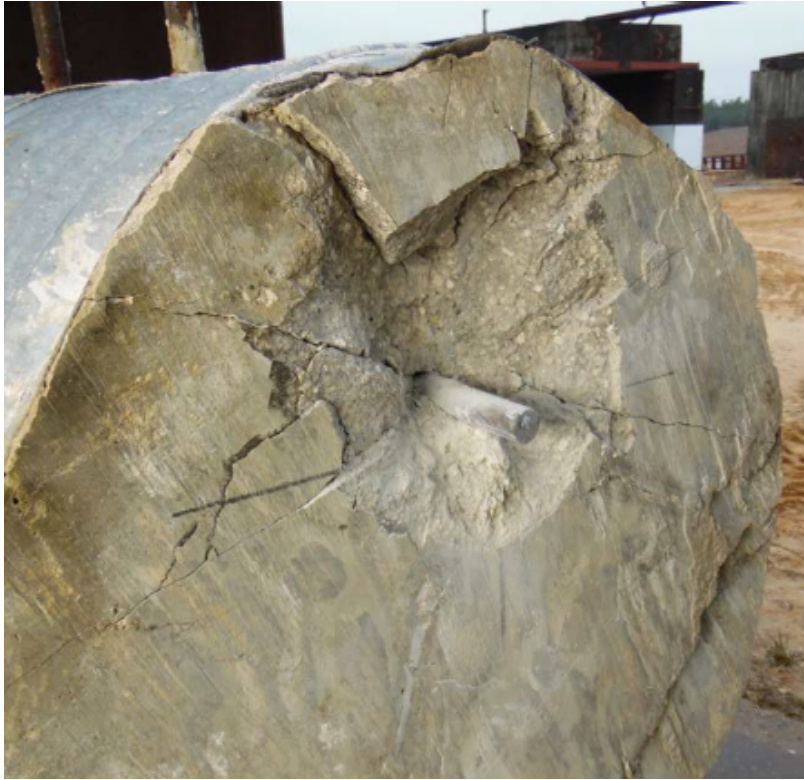
Figure 7. Graves' projectile is shown embedded within the concrete target. Note that the projectile is relatively intact.
