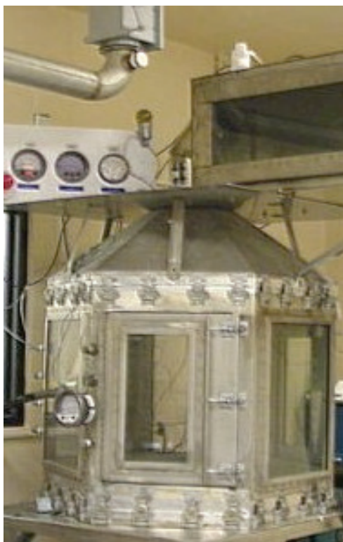
Figure 3. The 1000 L Rochester-style exposure chamber.
