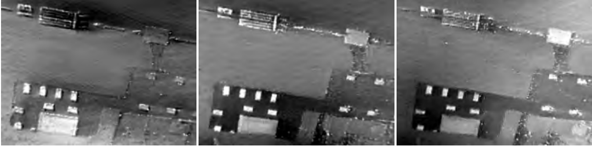
Figure 18: Camp Atterbury Dataset - Event Psuedo-Frames: Event-based frames from a similar time instance as that in Figure 17. From left to right, the values of n utilized are 0.05, 0.2 and 0.6.
