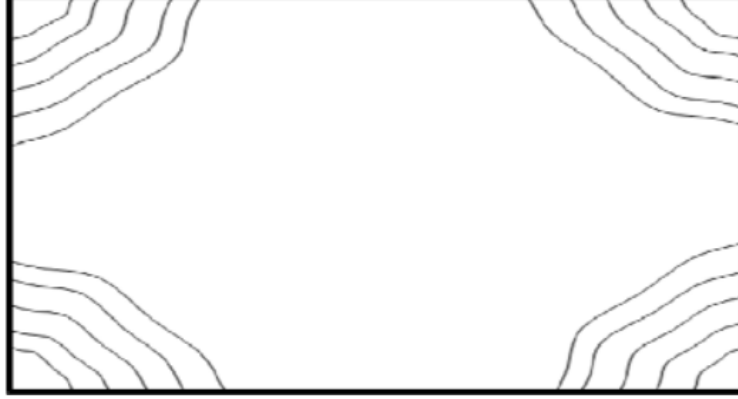
Figure 4: Geometric effects of spin coating photoresist onto rectangular substrates [3].
