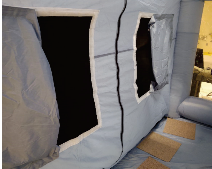
Figure 12. Large chamber wall partition with mesh panels opened halfway.
