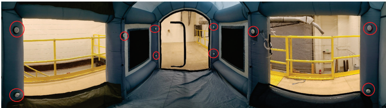
Figure 5. Panoramic view of installed air nozzles (circled in red) within small enclosure.
