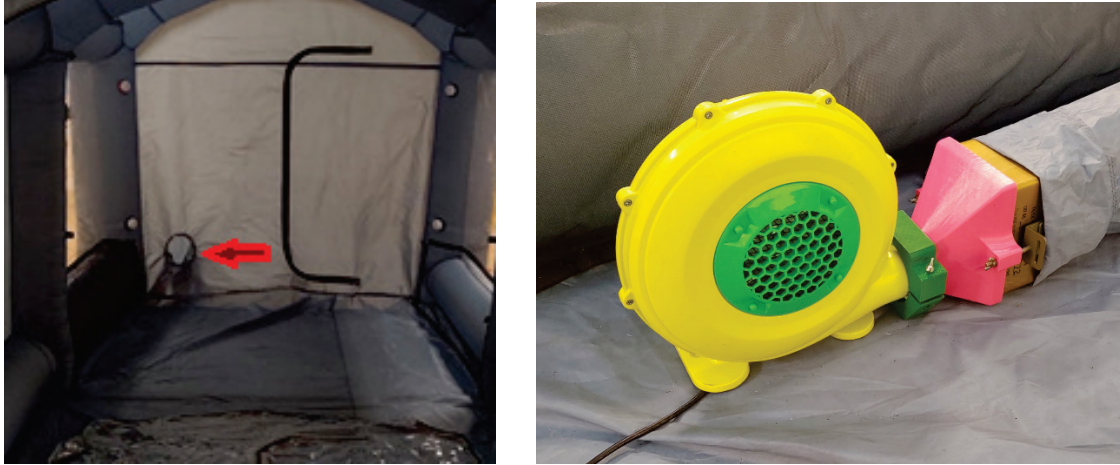
Figure 8. Small chamber exhaust location (left) and blower attached to exhaust system (right).
