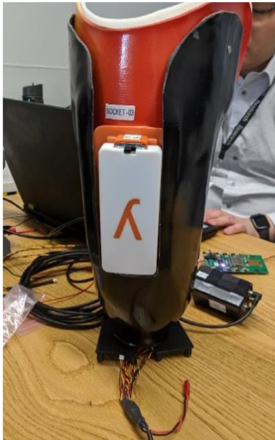
Figure 2-3. Photograph of the base-station affixed to the prosthetic socket. The entire system (implant and base station) is fabricated from off-the-shelf electronic components.
