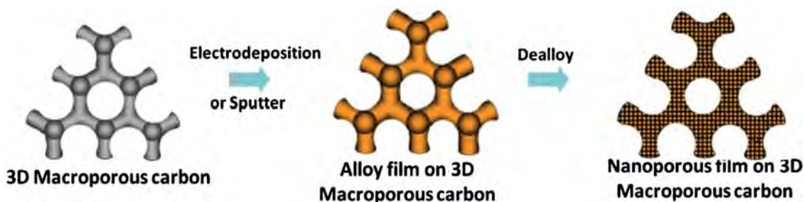
Figure 12. Schematic representation of the general process of depositing np metal films onto cellular structures. First, an alloy is deposited or sputtered onto a porous template. The alloy is then dealloyed so that the remaining material is a macroporous foam with a nanoporous coating. Reproduced from ref. [137] with permission of The Royal Society of Chemistry.
