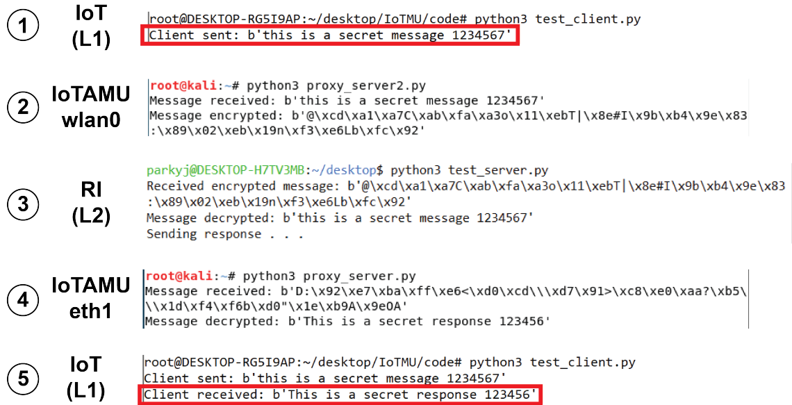
Figure 15: The flow of messages in the POC experiment testing IoTAMU’s encryption functionality.
