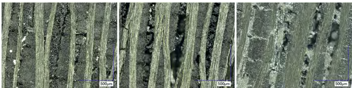
Fig. 3 Reflected-light microscopy generated images of classic (untreated) C/C (left), optimized C/C (middle), and optimized C/C-SiC (right) [50].
