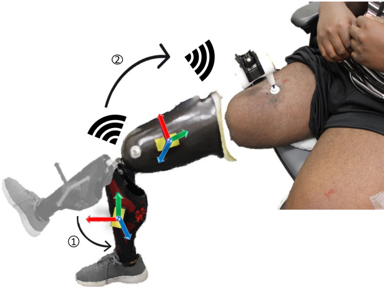
Figure 10. The participant was shown their prosthesis with wireless inertial measurement unit-based systems attached proximal and distal to the knee joint. They were informed that motion of the prosthesis, as detected by the wireless modules, was responsible for triggering the vibratory factor.
