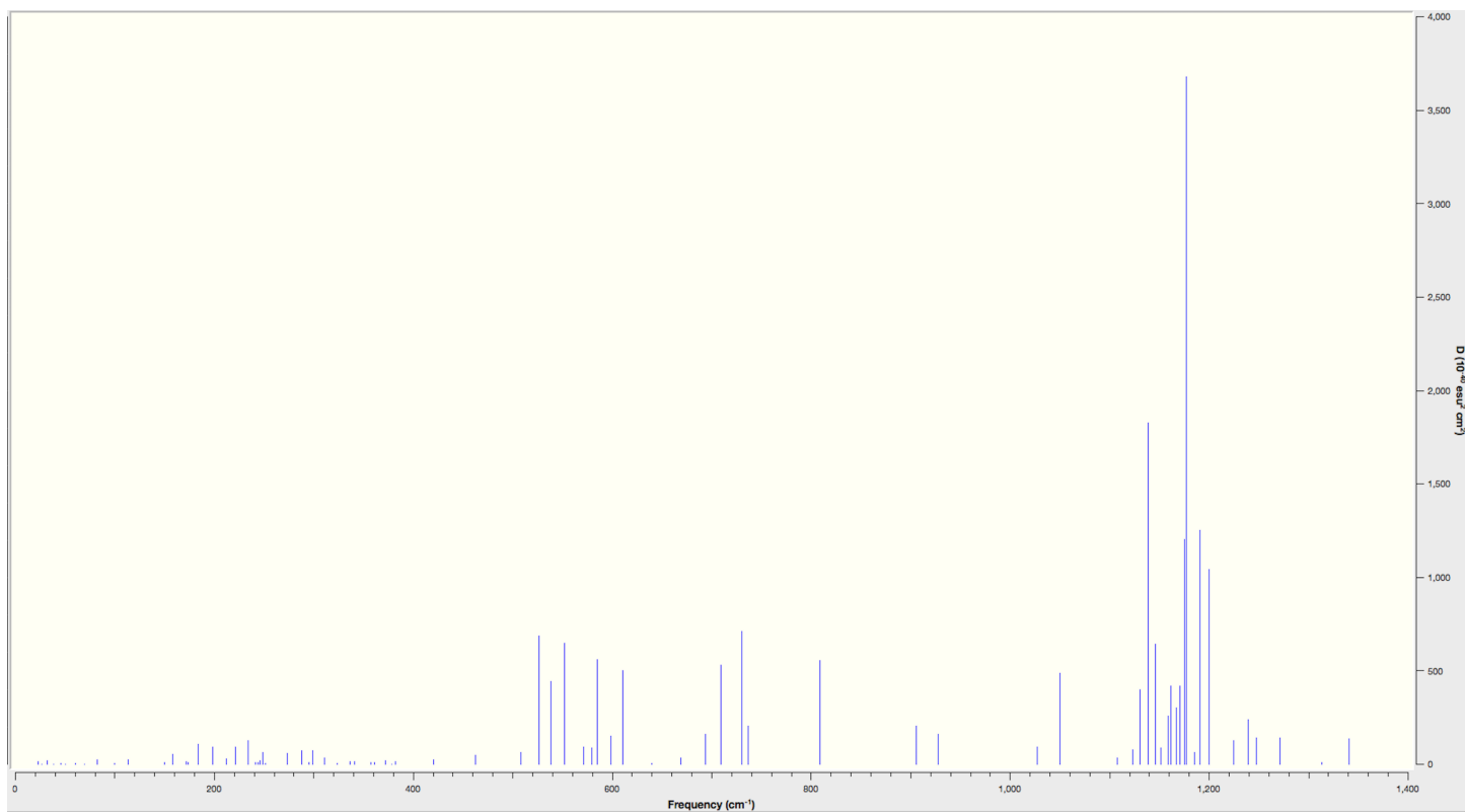
Figure 5A. DFT calculated IR spectra of C 8 F 17 -SO 3 . DMSO background (Energy: -2626.736028 Hartrees).
