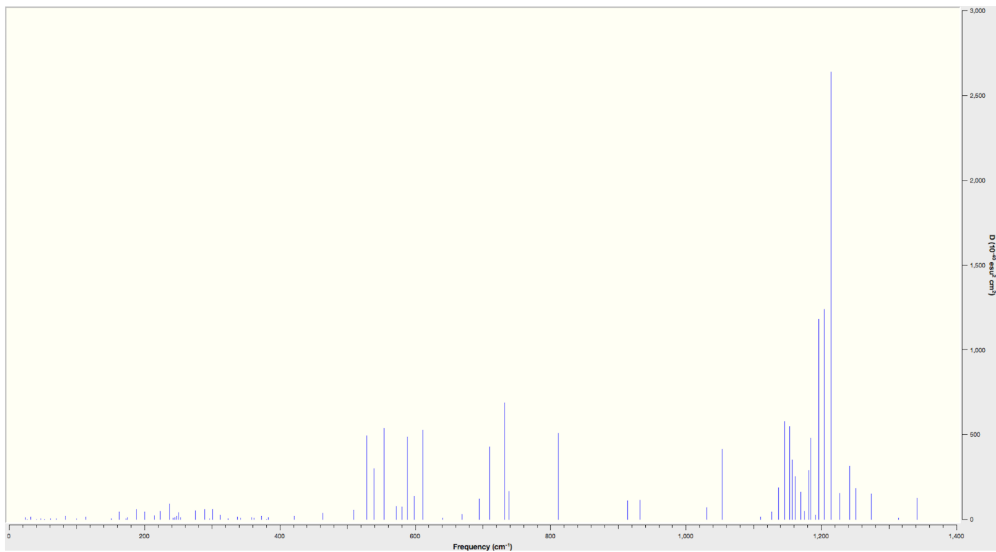
Figure 5C. DFT calculated IR spectra of C 8 F 17 -SO 3 . Toluene background (Energy: -2626.734457 Hartrees).
