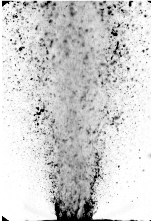
Fig. 5-Diffuse imageback-illumination imaging of spray from annular flow out of a laboratory-scale ( D=0.84 mm), OPA described by Fisher et al. [32,33]. The image is approximately 4.6 mm wide by 6.7 mm high. The flow rates were 0.4 g/s of air and 0.8 g/s of water. This flow had a GOR of 228 \text{ m}^3_{\text{air}}/\text{m}^3_{\text{water}} .
