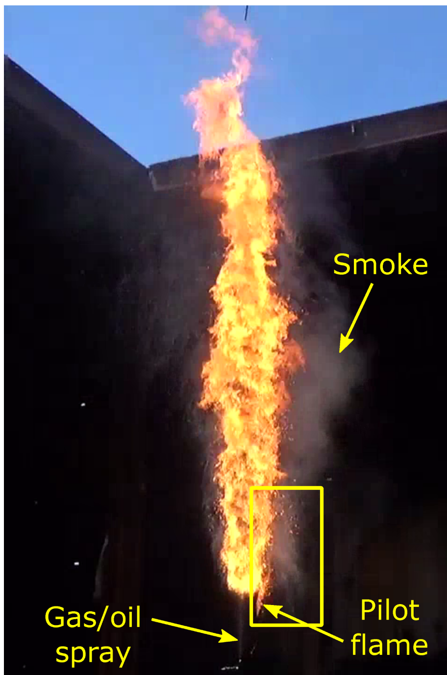
Fig. 10. Video/image of gas/oil spray flame for baseline condition (3 g/s gas, 16 g/s oil), recorded during a burn test on 14 May 2019. View is from the southeast corner of the chamber.
