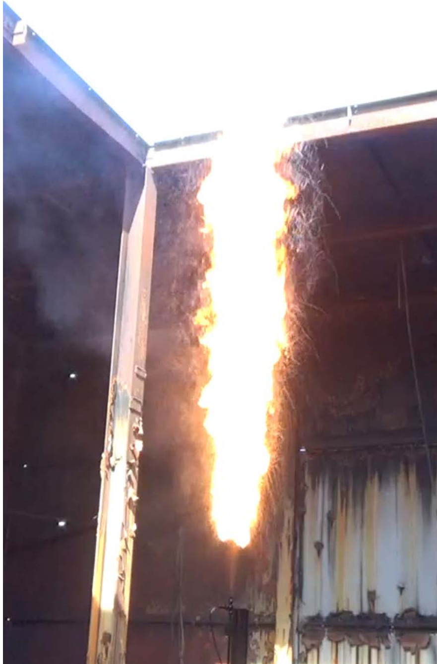
Fig. 50-Photograph of the burning spray plume operating with 3.0 g/s of 80:5:15% of \text{CH}_4 , \text{C}_2\text{H}_6 , and \text{C}_3\text{H}_8 and a blend of crude oils flowing at 16 g/s.
