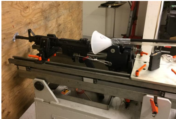
Figure 2 Weapon and sampling setup for BZTM, left inlet
