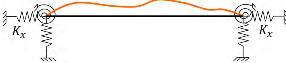
Fig. 50: Diagram of a flat beam with unknown axial stiffness terms K_x .
