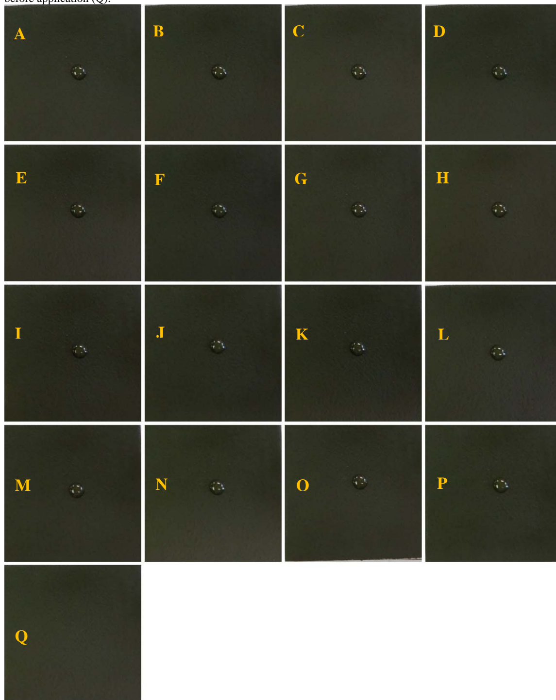
Fig. D1 — Paraoxon on ReColor S1. Images of the coating on a painted coupon at 0 (A), 0.5 (B), 1.0 (C), 1.5 (D), 2.0 (E), 2.5 (F), 3.0 (G), 3.5 (H), 4.0 (I), 4.5 (J), 5 (K), 10 (L), 15 (M), 20 (N), 25 (O), and 30 (P) min following application of the target and before application (Q).
