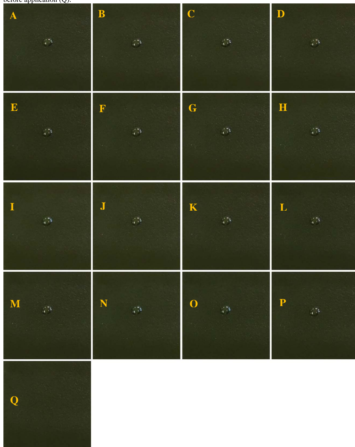
Fig. E2 — MES on ReColor S2. Images of the coating on a painted coupon at 0 (A), 0.5 (B), 1.0 (C), 1.5 (D), 2.0 (E), 2.5 (F), 3.0 (G), 3.5 (H), 4.0 (I), 4.5 (J), 5 (K), 10 (L), 15 (M), 20 (N), 25 (O), and 30 (P) min following application of the target and before application (Q).
