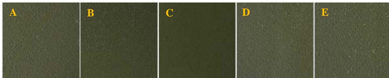
Fig. 1 — Images of a painted coupon (A), a Nanoskin treated coupon (B), a Wipe New treated coupon (C), a NeverWet treated coupon (D), and a NanoWax treated coupon (E). [1]
