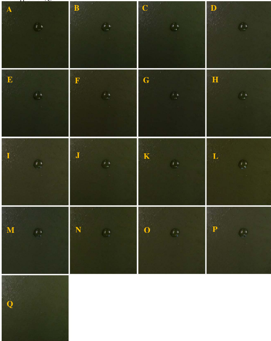
Fig. K3 — DMMP on ReColor SC3P. Images of the coating on a painted coupon at 0 (A), 0.5 (B), 1.0 (C), 1.5 (D), 2.0 (E), 2.5 (F), 3.0 (G), 3.5 (H), 4.0 (I), 4.5 (J), 5 (K), 10 (L), 15 (M), 20 (N), 25 (O), and 30 (P) min following application of the target and before application (Q).
