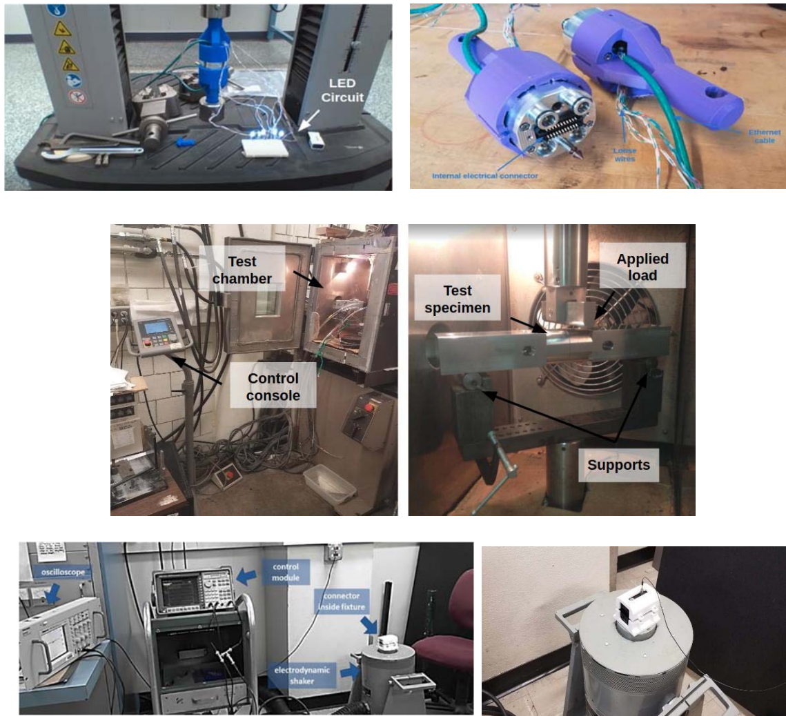
Figure 38 Top: Axial Pull Tests, Middle: 3 point Bending Tests, Torque, Bottom: Vibration Testing
