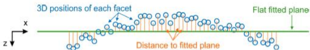
Figure 5.11 Schematic of the best fit plane method used by Istra 4D to estimate the shape of the plate.
