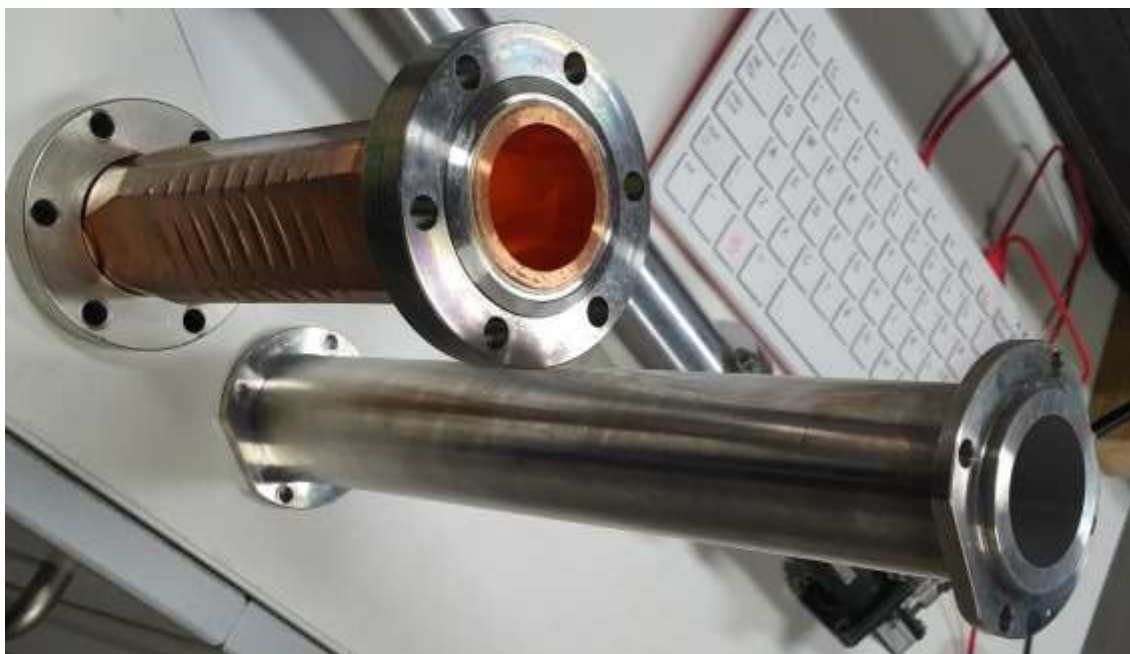
Figure 24 Comparison of corrugated and elliptical approaches to the circular polariser
