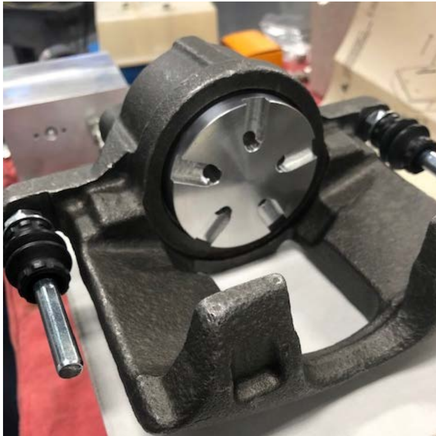
Figure 5. Caliper and Machined Piston
