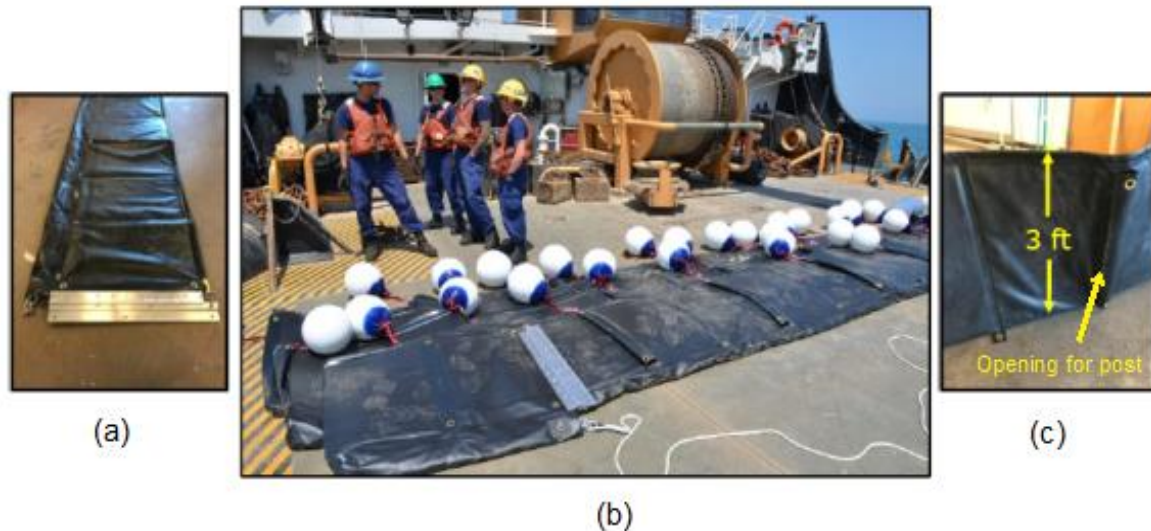
Figure 7. Offshore mitigation system prototype.
