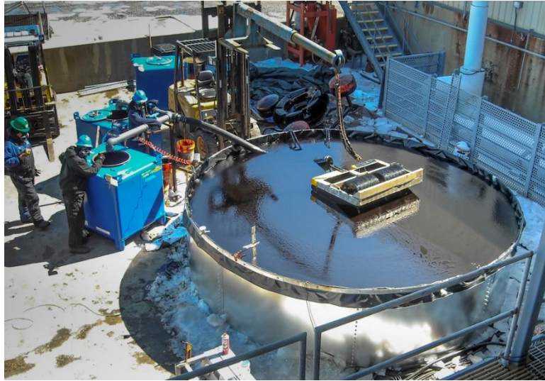
Figure 3. Skimmer test with dilbit in Ohmsett's fresh water tank.
