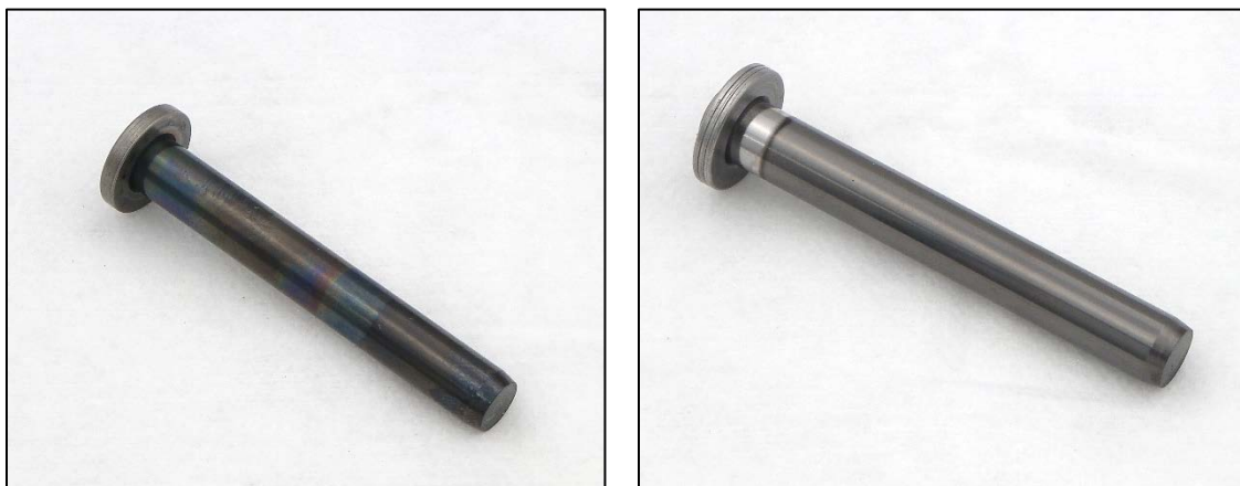
Figure 28. C7 HEUI Injector Plunger (CYL#4 shown left, NEW shown right)
