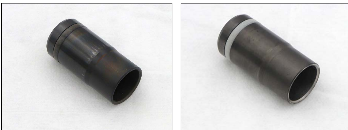
Figure 27. C7 HEUI Injector Plunger (CYL#5 shown on left, NEW shown on right)
