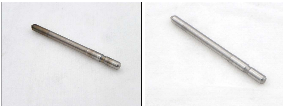
Figure 31. C7 HEUI Injector Needle (CYL#4 shown left, NEW shown right)
