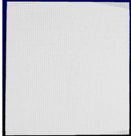
Figure 17. X-ray CT scan of test sample 2.1. The lack of black dots indicates the lack of porosity in the material [15].
