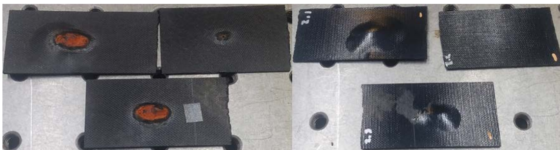
Figure 34. Top Left, sample 2.1 nanotube alignment along the long axis of the beam. Top right, sample 2.2 nanotube alignment orthogonal to the long axis of the beam. Bottom, sample 2.3 nanotube alignment 45 ° to the long axis of the beam.
