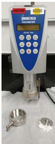
Figure 11. LVDV-II+Pro Brookfield viscometer with a CPE40 plate.
