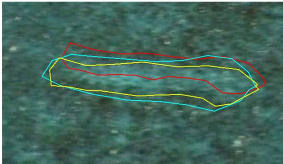
Figure 52. Three snorkeler-derived GPS measurements of the area of damage of the Evening Star ship grounding (red, blue, yellow outlines) overlain on aerial imagery of the scar taken from Google Earth.
