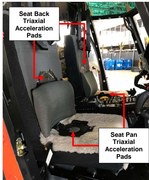
Figure 3. Acceleration Pads mounted to Seat Pan and Seat Back at Pilot/Copilot stations. Accelerometer Pack attached to lower left seat rail at both stations
