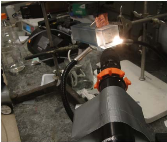
End-on images of coalesce screens under aerosol exposure
