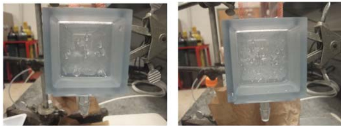
End-on images of coalesce screens under aerosol exposure
