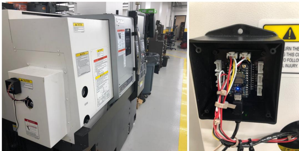
Figure A1. Photon-based reconfigurable retrofit kit sensor package at GT.
