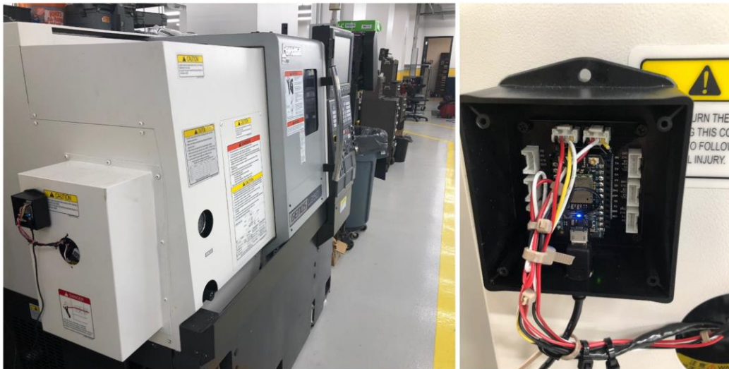
Figure 6. Photon-based reconfigurable retrofit kit sensor package at GT.
