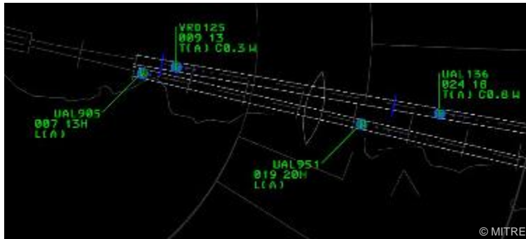
Figure 5-11. Case B: Separation Violation Between UPS905 and UAL951 at the Time of Occurrence
