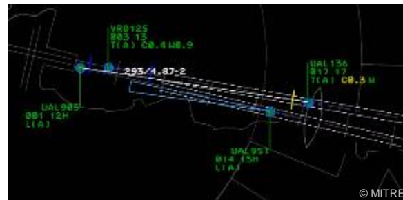
Figure 5-10. Case A: Example Separation Violation Between UPS905 and UAL136
