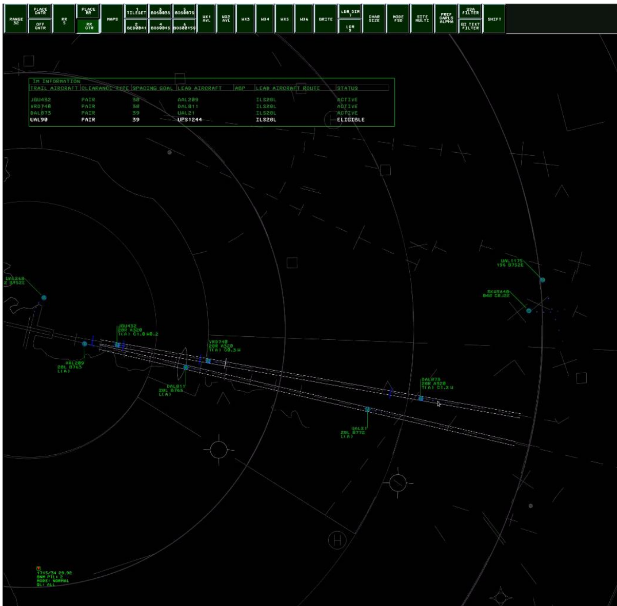
Figure 4-1. STARS Display used in the HITL Experiment (with IM PA Display Features)
