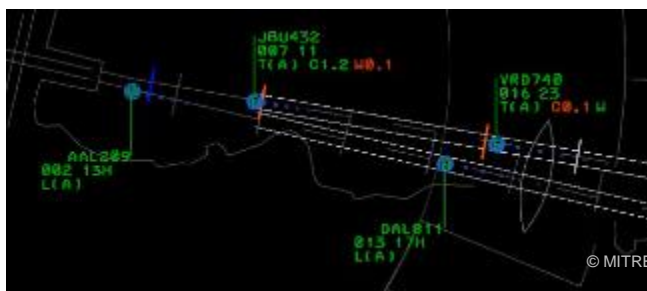
Figure 5-18. Case E, Occurrence 12: Separation Between JBU432 and DAL811 at the Time of the JBU432 Caution Alert
