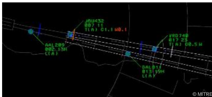
Figure 5-17. Case E, Occurrence 11: Separation Between JBU432 and DAL811 at the Time of the JBU432 Caution Alert
