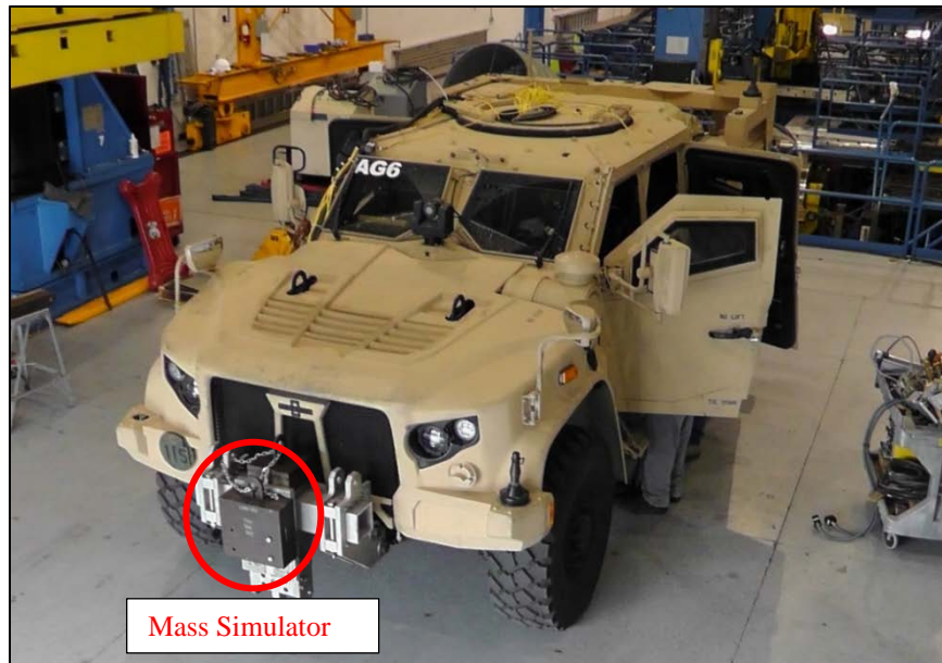
Figure 11. Test vehicle restraint bracketry with mass simulator.
