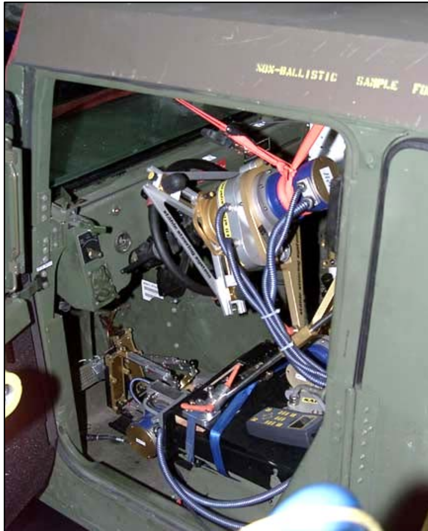
Figure 8. RWS autopilot mounted in a HMMWV.
