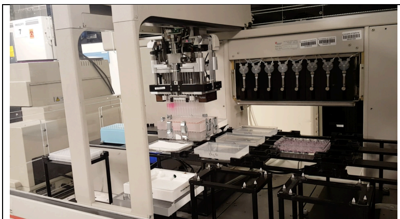
Figure 1. PMF setup in the Molecular Shared Screening Resource, UCLA's high throughput screening core facility. Photo shows 96-well pipette head loading samples into the PMF device top plate.
