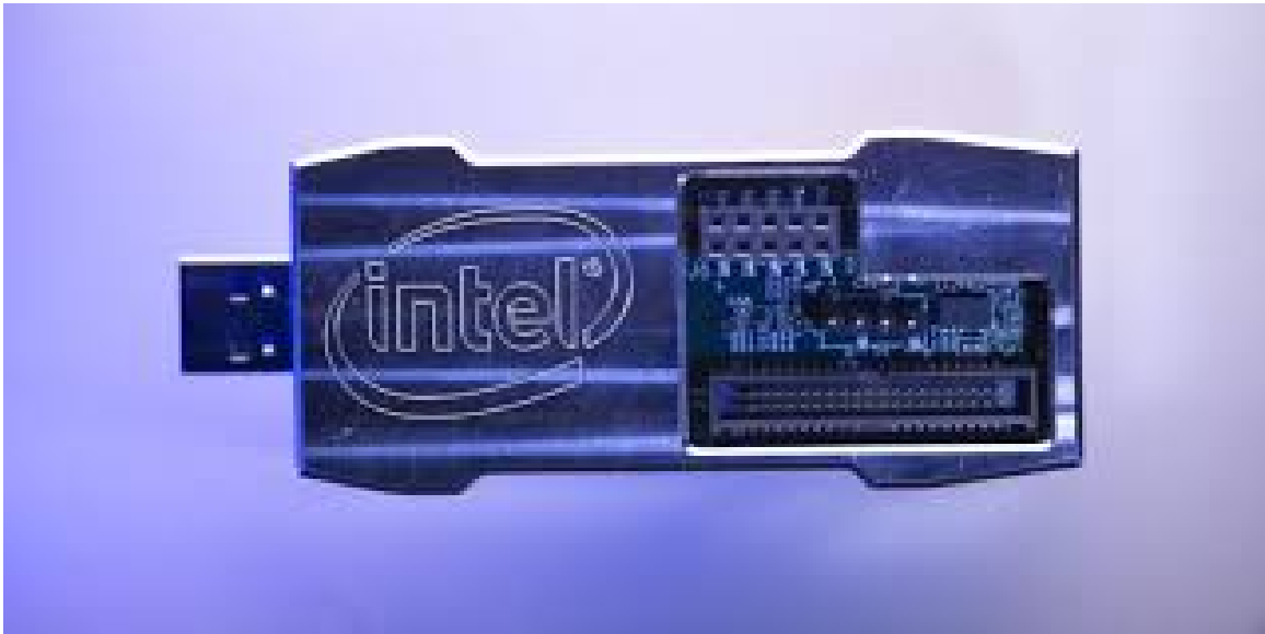
Figure 2.2: Intel Loihi Kapoho Bay USB, picture taken from [2]
