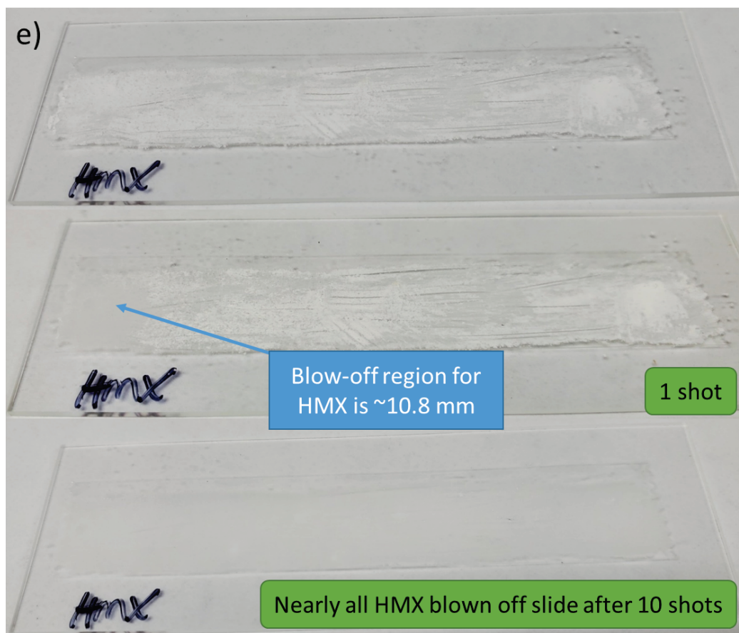
Fig. 2 Prepared sample slides, including a) the blank tape substrate, b) TNT, c) TATB, d) RDX, e) HMX, and f) CL-20. The first slide in each series consists of the as-prepared slide; subsequent images in each series show the slide after one or more laser shots. (continued)
