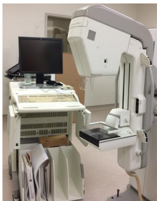
Figure 5: A full field digital mammography system (Senographe 2000 D, GE Healthcare) was installed in our lab to construct the prototype trimodal mammography imaging system.
