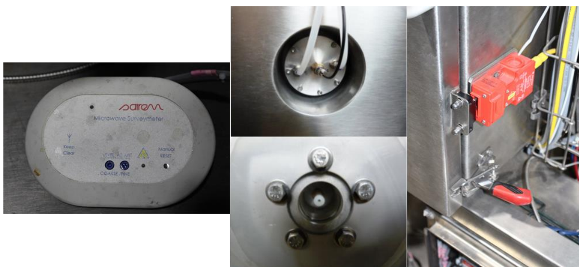
Figure 3.3. From left to right: The microwave leakage detector, fibre optic arc detector behind a quartz window and the MW door safety interlock.
