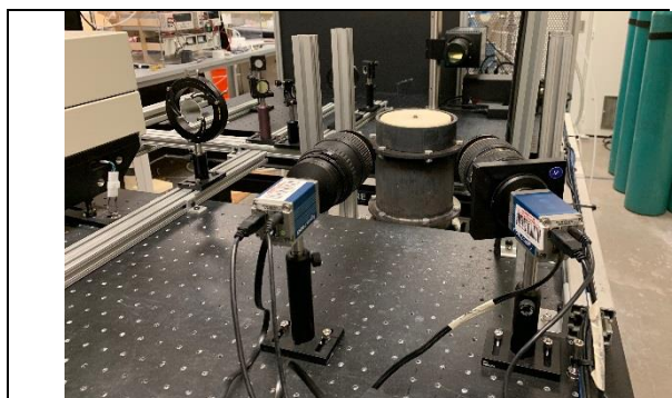
Figure 2.3.2 – Stereo-PIV / HCHO-PLIF experiment implemented at Professor Narayanaswamy's laboratory at NC State University.
