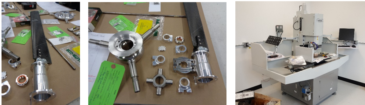
(a) isolated blade (b) blade and gimbal hub (c) 4-axis Tormach mill Figure 2. Tiltrotor blade shown with parts of the new gimballed hub.
