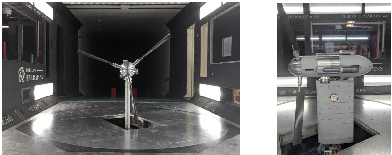
Figure 10 Blades installed (twisted blades shown) and stress tested from 900-2400 RPM on the Maryland Tiltrotor Rig at the Glenn L Martin Wind Tunnel in September 2019; wind-off conditions; 2400 RPM equals tip Mach number of 0.6; at the time, only 2 identical swept blades could be fabricated, hence these were not tested on MTR.
