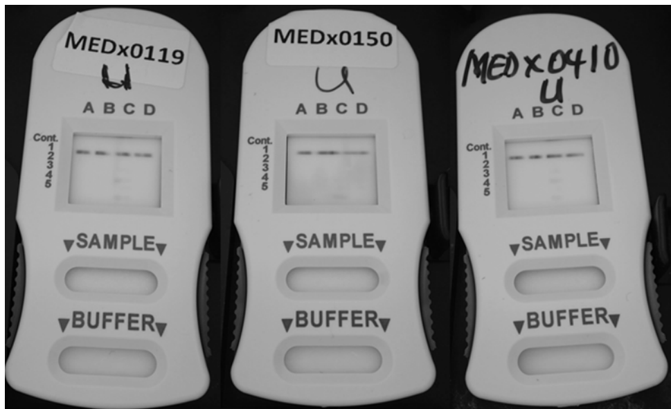
Fig. 5—Examples of MEDx urine tests called positive for BURK by Deki reader, where lanes have shifted within the test window.
