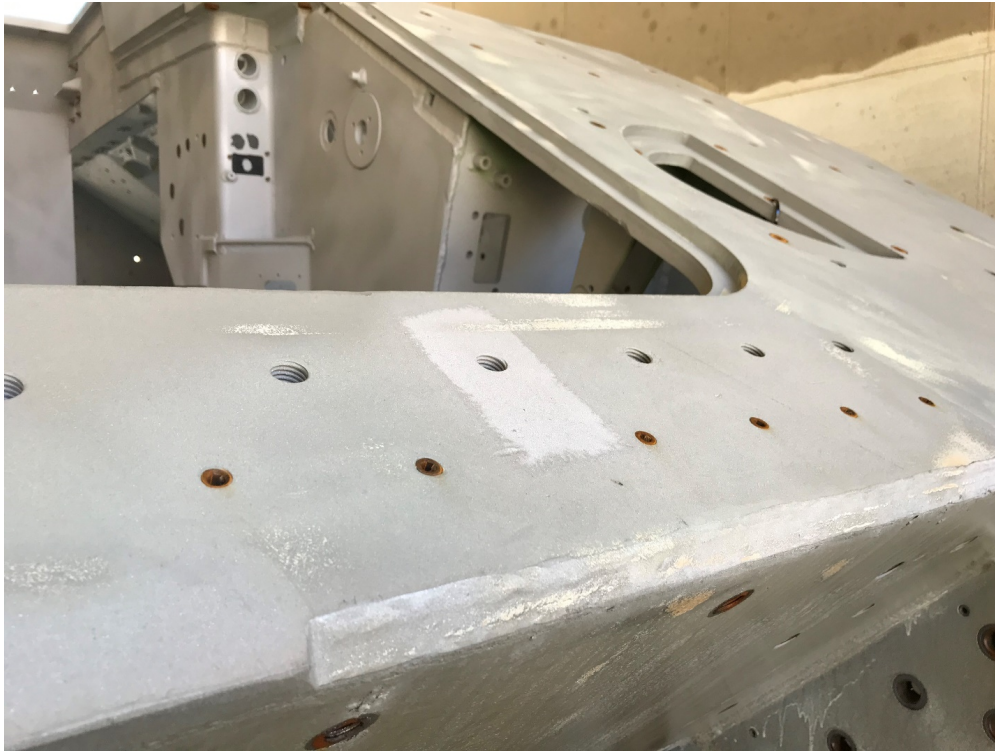
Fig. 9 Finish achieved with LVLP spray gun. Note color change on Al where tape was removed.
