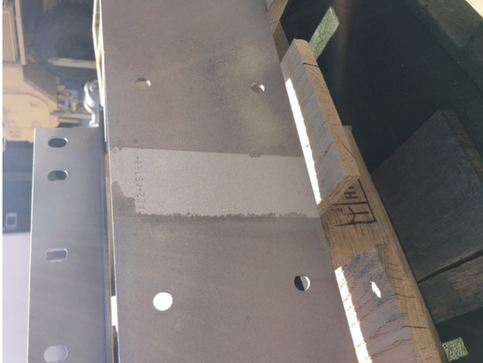
Fig. 10 Color change on steel where tape was removed
