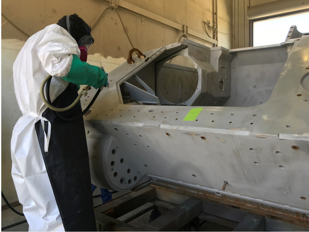
Fig. 5 Application with LVLP. Note masking tape to witness color change.
