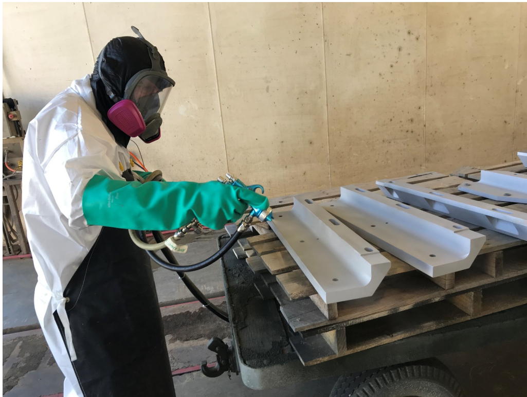
Fig. 8 Spray application of Bonderite M-NT 7400 onto aluminum sponson parts
