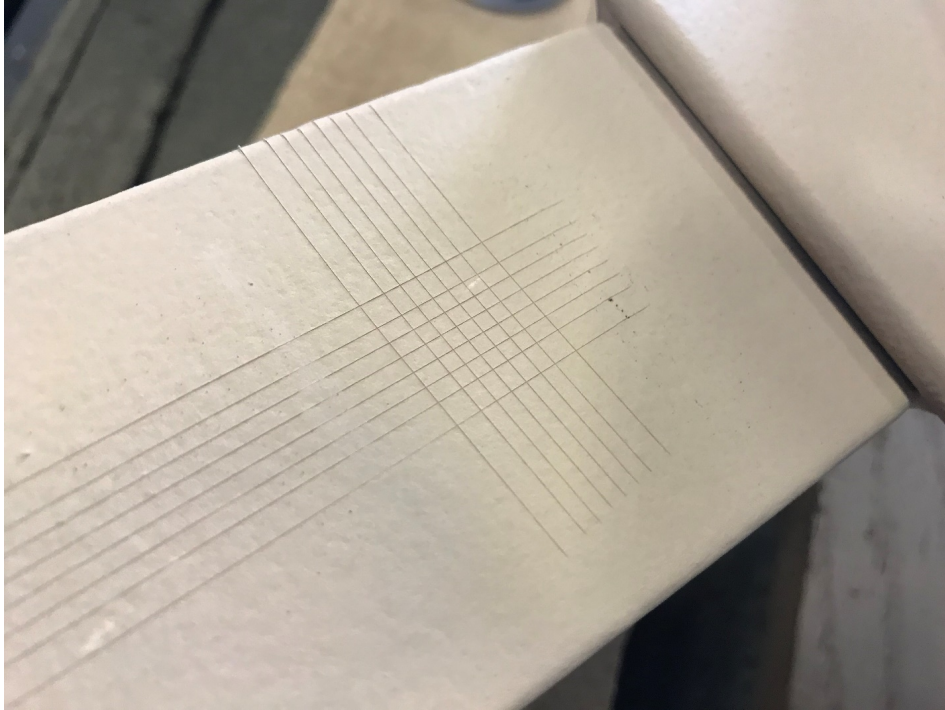
Fig. 13 Adhesion test on welded steel frame, 5B
