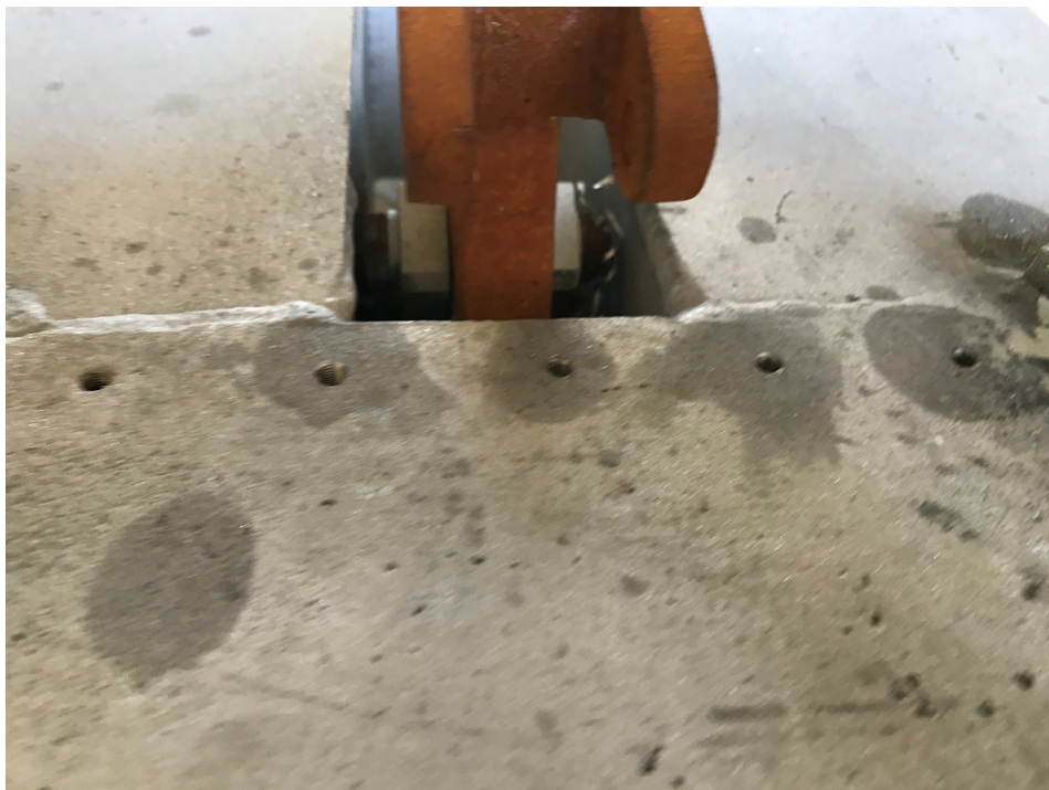
Fig. 12 Hull not processed with Bonderite M-NT 7400 because of oil contamination
