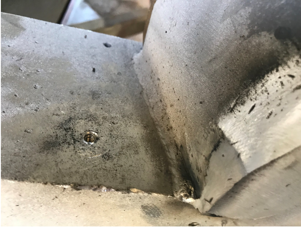
Fig. 11 Welded Al assembly not ready for paint application because of oil and weld spoils
