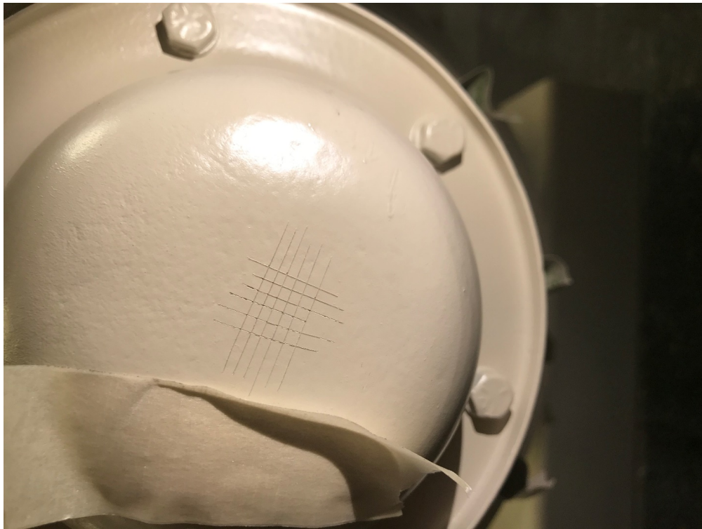
Fig. 15 Adhesion test on axle assembly, 5B
