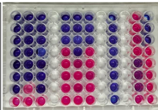
Figure 2. Broth microdilution assay in triplicate. Columns 1-3; DAN-1-13 serial microdilution. Columns 5-7; DAN-1-71A serial microdilution. Column 9. Blank (culture medium only). Column 11. Negative control (medium and inoculum); in the last four wells, DMSO was applied to assess solvent-related toxicity. Column 12. Positive control (Vancomycin microdilution)
