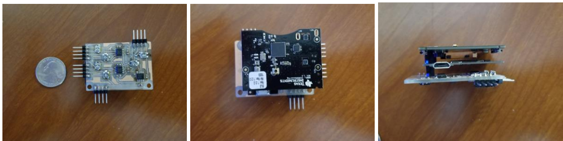
Figure 17. Amplifier board with Sensor Tag & Debugger
