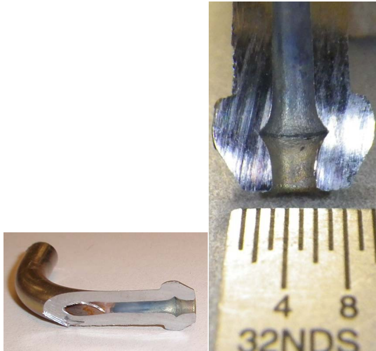
Figure 10. Fuel line reverse engineering and dimensional analysis
