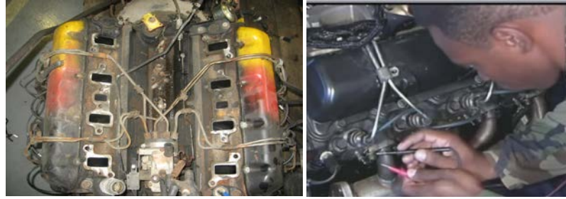
Figure 6. High Mobility Multi-Purpose Wheeled Vehicle 6.2L repair environment
