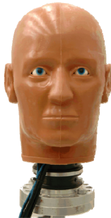
Figure 1: The FOCUS headform is designed to predict the risk of eye and facial injuries, and was particularly designed to help evaluate facial and ocular protection.
