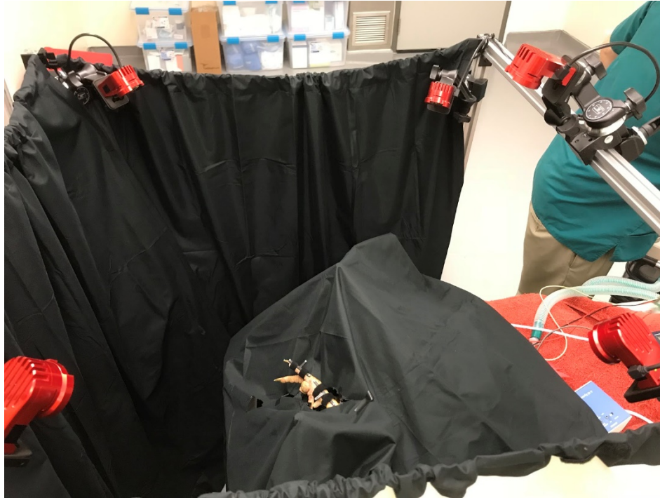
Figure 10: Motion capture environmental with chicken foot and retroreflective markers to measure the range motion.
