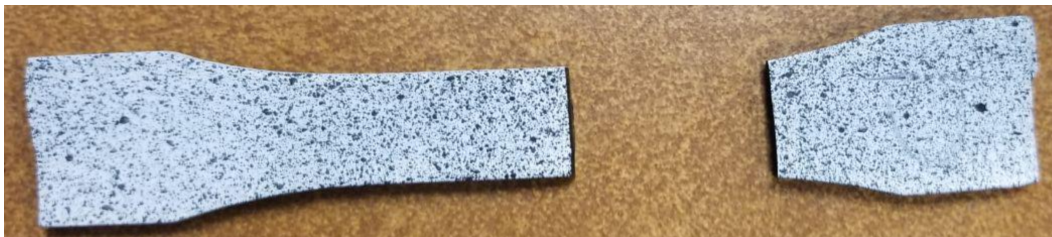
Figure 24: Non-fouling coating sample fracture
