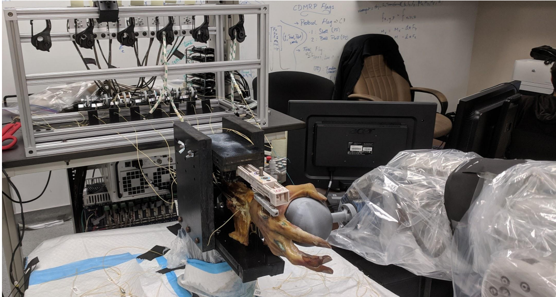
Figure 1: Image our actual experimental setup shows the AdeptSix 300 robot in the foreground, with the instrumented ball mounted to its end-effector. It is covered in plastic to safeguard it from human tissue contamination. The hand is mounted to our setup using the Agee WristJack with its tendons actuated by the frame-mounted motors in the background. CamJam adjustable rope anchors are used to passively tension the interosseous and Abductor Pollicis tendons.
