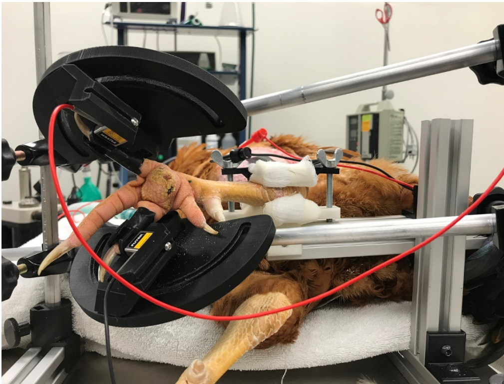
Figure 8: Left pelvic limb of the chicken rigidly fixed and mounted with force transducers interfacing the splinted lateral and medial toes to measure toe tip forces and observe the interplay between the coupled toes.
