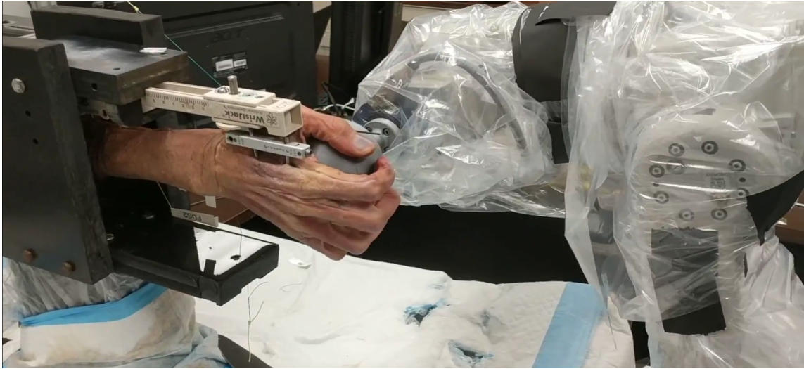
Figure 6: The cadaver hand specimen is mounted to our setup. The active tendons are wired to are motors which simulate muscles. The passive tendons are anchored to provide tension for posture. Then the instrumented ball on the robotic arm is used to test grasp.
