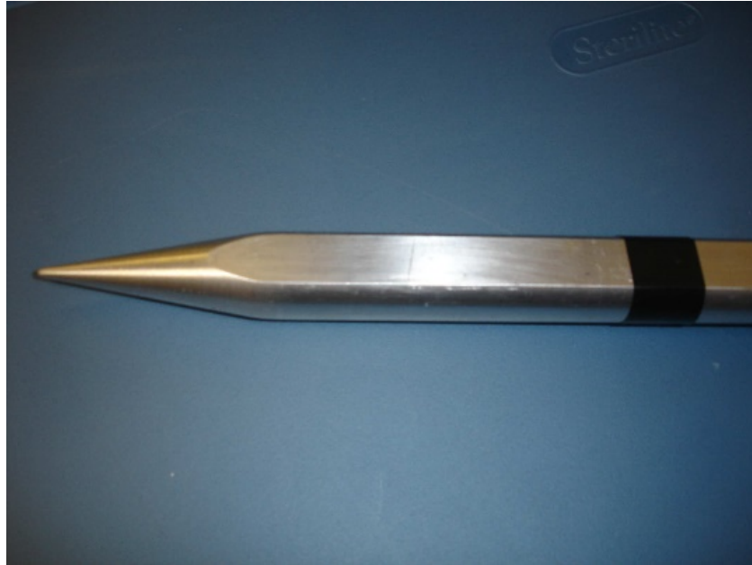
Fig. 5 Electrical tape wrap on sensing element 3
