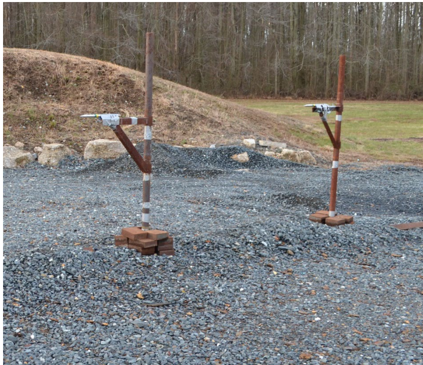
Fig. 7 Array of pencil probes mounted in a real experiment
