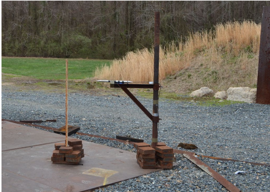
Fig. 8 Sacrificial pole protecting the pencil probe
