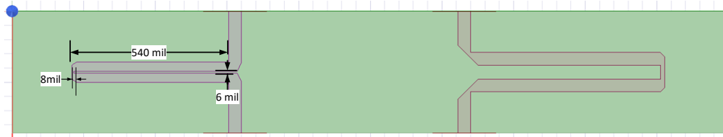
Figure 22: Layout and dimensioning of 45deg phase shifter
