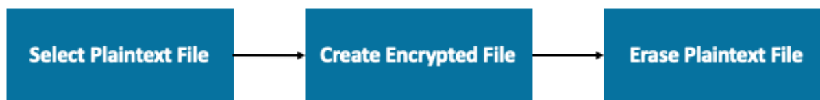
Figure 10: Ransomware File Encryption Workflow
