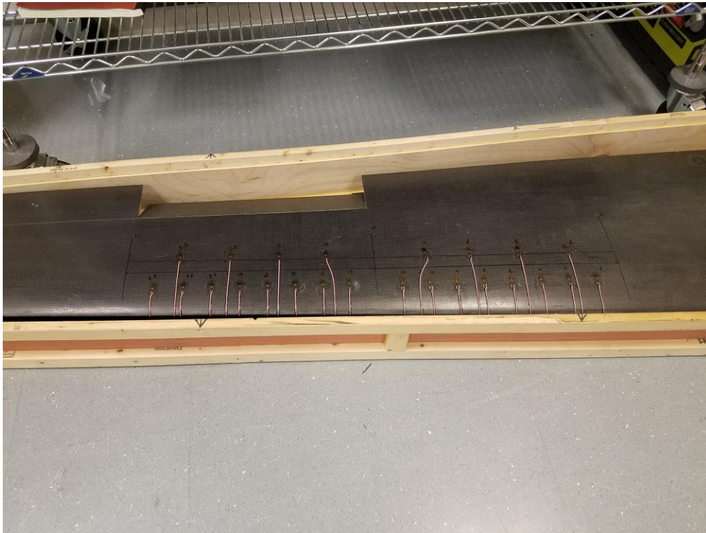
Figure 8. Fully assembled wing with strain gauge layout.
