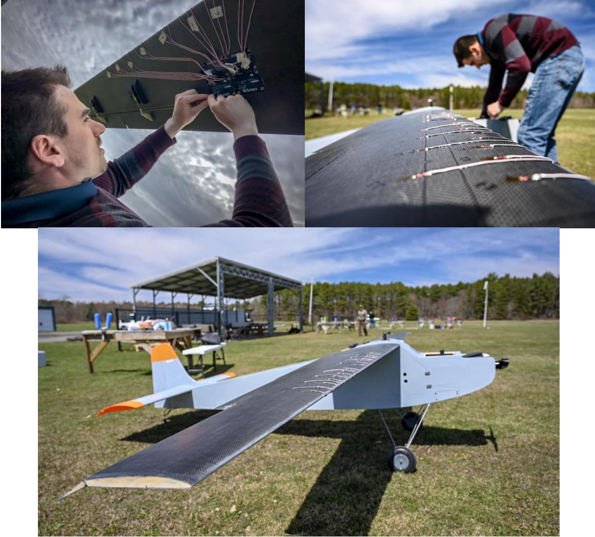
Figure 18. (Top) Pre-flight assembly of the aircraft sensor board and checkout of the aircraft power system. (Bottom) Fully assembled flight-ready aircraft system.
