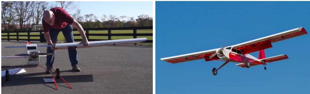
Figure 2. A giant Telemaster RC aircraft system was chosen as the basis around which the testbed aircraft was developed. This aircraft system provided a large enough wing planform to house the required sensors and avionics and enabled custom wings to be easily swapped out within the same flight test.
