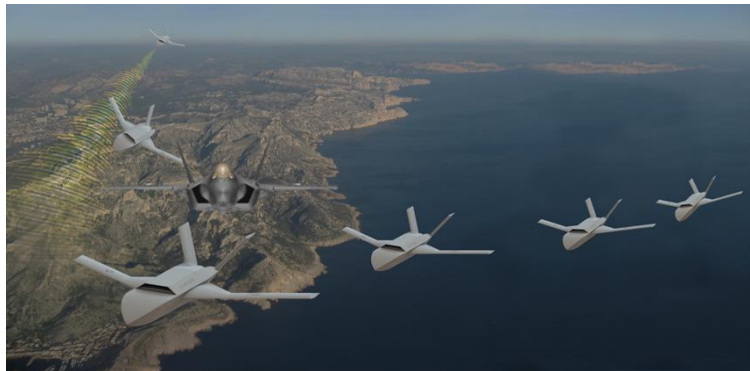
Figure 1: The Aurora LCAAT/Loyal Wingman concept. LCAAT vehicles must operate autonomously in complex environments and are designed for a cost per capability metric, thereby requiring the reduction of subsystem reliabilities. Vehicle self-awareness therefore will play a key role in the mission performance of these systems.
