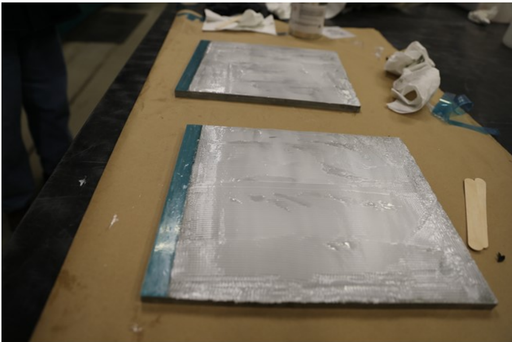
Fig. 14 Representative example of the manual spreading of a 1-component paste adhesive
