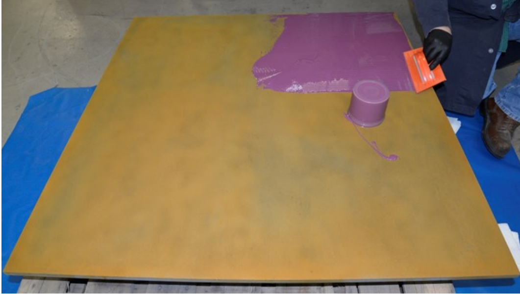
Fig. 12 Application of a 2-component paste adhesive to a section of RHA steel. Note: The RHA steel was grit blasted and pretreated with a commercially available non-chromate wash-primer prior to bonding per TT-C-490G. 58
