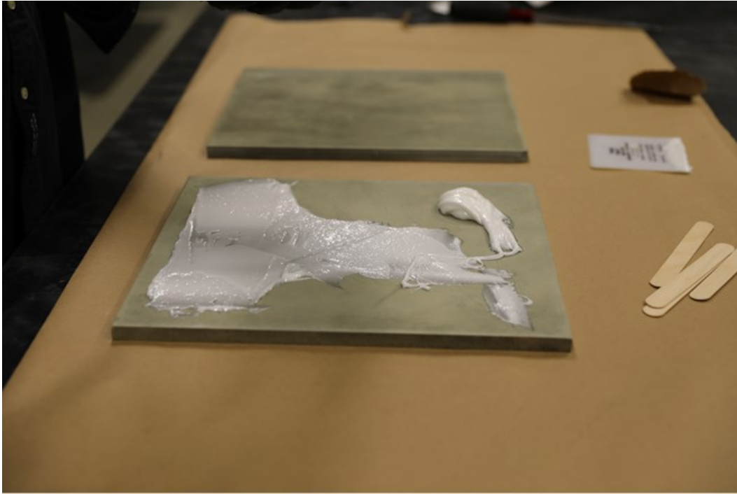
Fig. 13 Representative example of the manual application of a 1-component paste adhesive to 300- × 350-mm 2024-T3 Al plates for required for the Tier III: Crack extension test
