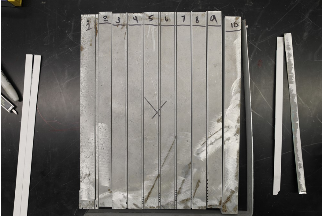
Fig. 5 Post machining of the bonded 300- × 350-mm 2024-T3 Al for Tier III crack extension testing will yield 10 individual samples
