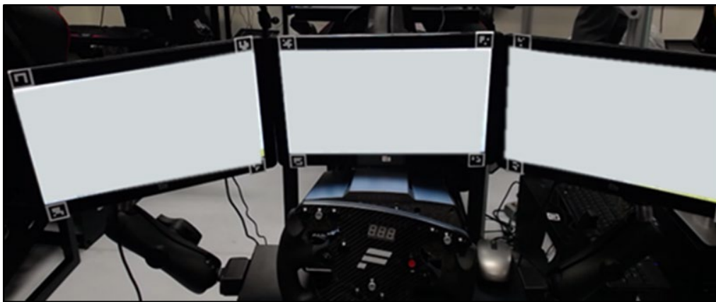
Fig. 2 Example crew station with three touchscreen displays and vehicle controls that allow participants to interact with the simulated manned and robotic vehicles
