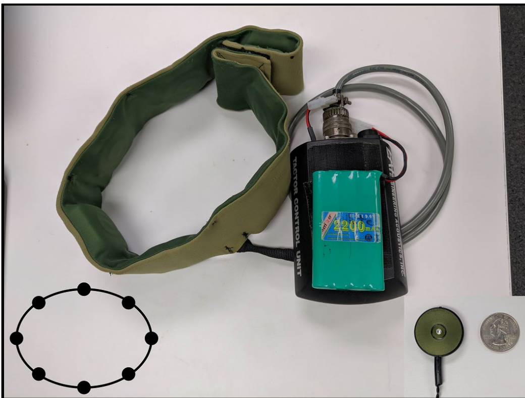
Fig. 6 A tactile belt is used as part of the Transparent WMI condition to provide cuing to crew members whenever they encountered an environmental threat. Diagram (bottom left) depicts factor position in the belt.
